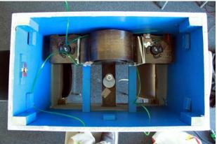
The two to four inducer speakers, breath sound into the clocks wood to witch new stethoscopes are linked.
